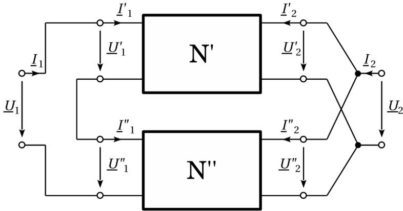
$$\begin{aligned} \underline{I}_1 &= \underline{I}'_1 = \underline{I}''_1 & \underline{U}_1 &= \underline{U}'_1 + \underline{U}''_1 \\ \underline{U}_2 &= \underline{U}'_2 = \underline{U}''_2 & \underline{I}_2 &= \underline{I}'_2 + \underline{I}''_2 \end{aligned}$$
